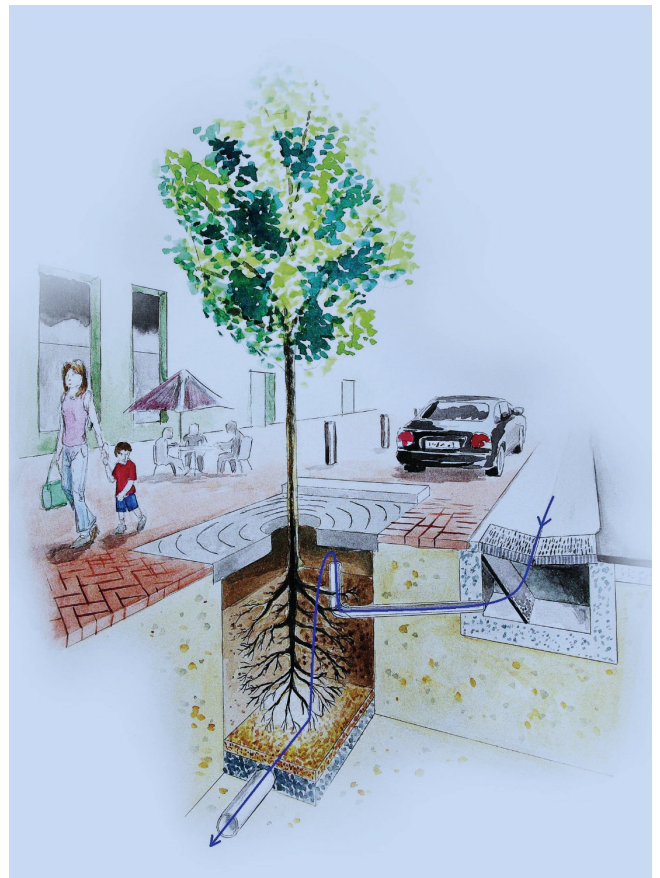
Coronation St, Hornsby – Tree pit biofilter (artwork by Stephen Pym)
